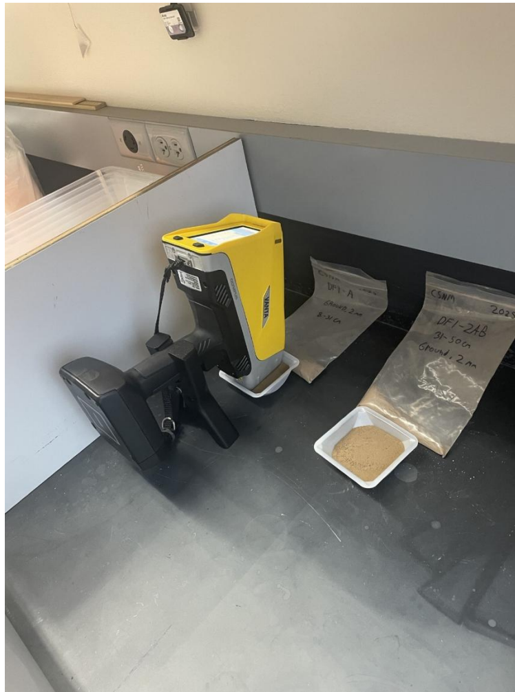
Figure 11: Geochem 3-Beam analyzer testing the samples in the lead cage at OSU.
