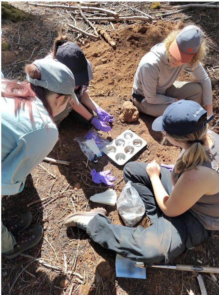
Figure 4: OSU students observing field technique of pH in NaF, an indicator of poorly crystalline or short-ranged order minerals in soils. This test was not necessary for the completion of the project, as these soils were dominated by phyllosilicates, but it was a simple test to demonstrate soil chemistry in the field for student understanding.
